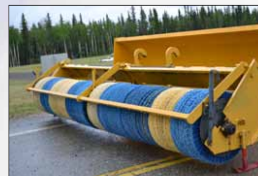
The "Scruncher" keeps breaking action optimum for small aircraft on the East Ramp at PAFA
